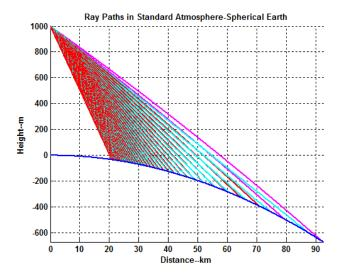
defines the visible horizon. The atmosphere extends the visible horizon from source at a fixed height. The practical ramifications are clear. For example, one is trying to aim laser at a point on the ground, the appropriate launch angle must be determined. Ray tracing provides a practical way to calculate an appropriate set of pointing directions; moreover, propagation anomalies such as ducting can be investigated as well.
